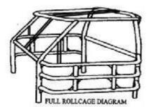
bar that goes up to the halo. One horizontal bar from extra bar to B bar, does not have to be 1 1/4"
